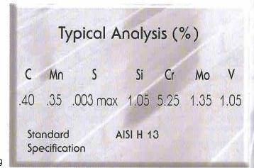
**SF-H 13 ESR** is made by the "densified method" specially designed to forge tool steel with improved isotropic properties, higher strength and greater freedom from internal discontinuities. Those characteristics combined with a minimum reduction ratio of 5 to 1 enhance the density of the steel and provide great homogeneity.
